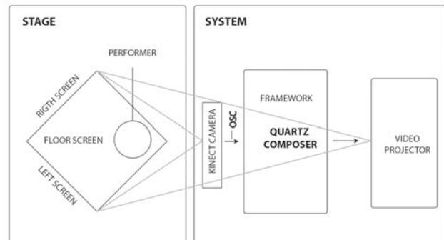
Figure 2. © João Beira. System architecture and physical setup
